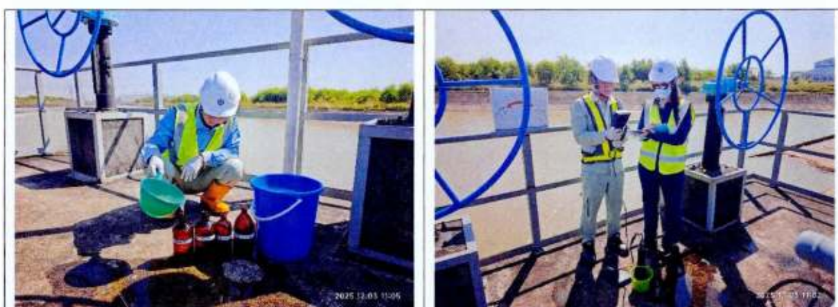
Surface water sampling and onsite measurement at SW-8
