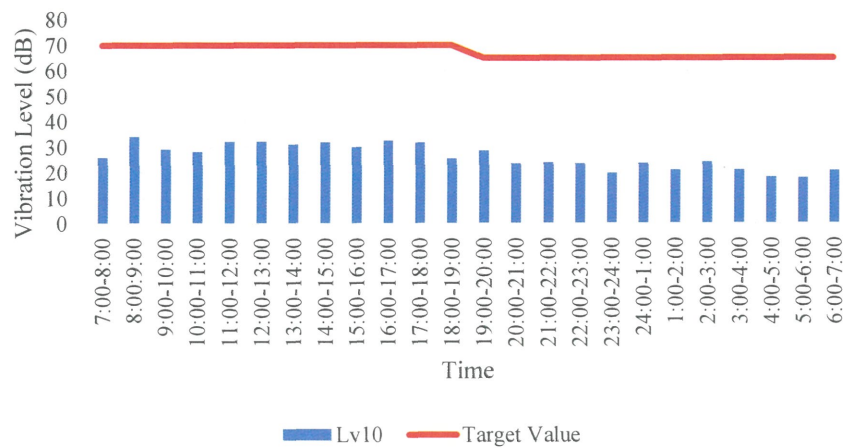
Figure 2.4-6 Results of Vibration Levels ( L_{v10} ) Monitoring at NV-3
