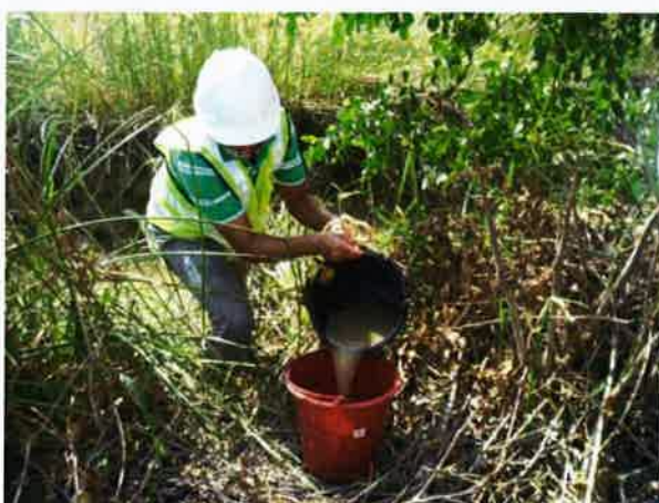
Surface water sampling and onsite measurement at SW-3
