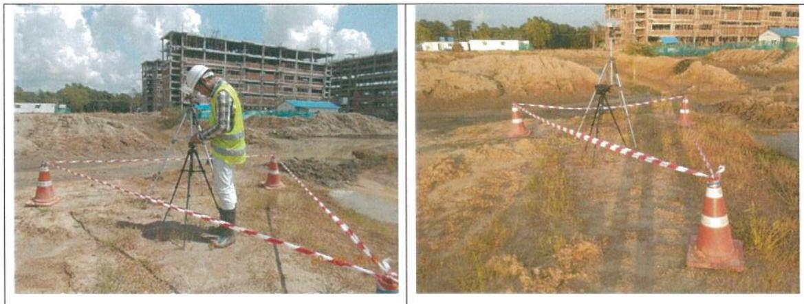
Figure 4. Noise and vibration monitoring at NV-2.
